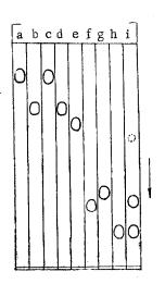
Scheme of the chromatogram. System: butan-1-olethanol-water-ammonia (40:10:49:1). Chromatography for 18 hr. "B" paper of the Volodarskii Leningrad No. 2 mill: a) D-glucose reference sample; b) D-fucose reference sample; c) D-glucose from glycoside Z; d) D-fucose from glycoside Z; e) 3-methyl-D-glucose; f) 2, 3, 4-trimethy1-D-glucose; g) 2, 3, 6-trimethyl-D-glucose; h) 2, 3, 4, 6-tetramethyl-D-glucose; i) hydrolyzate of methylated glycoside Z.
